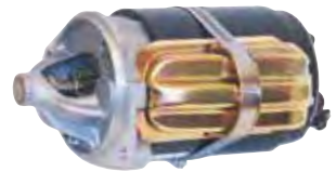
18-6276 STARTER Replaces: 984536, 988013 • 12 Volt • CW Rotation • Threaded Top Hole in Housing • 460 Ford, OMC King Cobra
