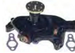
18-3583 CIRCULATING WATER PUMP (Bi-Directional) Replaces: 60658, 8503991, 17437 For: GM V-6 & V-8 engines with stamped steel timing covers.
