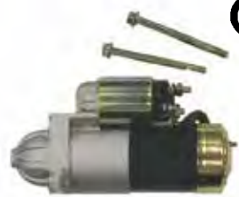
18-5913 STARTER (Clockwise) Delco permanent magnet gear reduction 2 bolt starter 12V - 11 Tooth - Offset bolt pattern. Fits: Chevy Engines with 14" flywheels. 1.7 KW Replaces: 3854751 SAEJ1171 Replacement Solenoid: 18-6287
