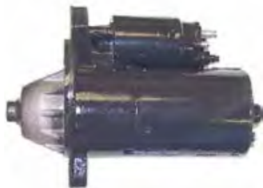
18-5920 STARTER Replaces: 3854190 Permanent magnet starter Replacement Solenoid: 18-6291 For: 5.0 & 5.8 litre Ford engines
