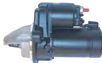
18-6292 STARTER Replaces: 872241 • Inboard • Gear Reduction Starter • Permanent Magnet, 12 Volt • CW Rotation • Aluminum Pinion Housing w/2 Threaded Mounting Holes Fits : Volvo Penta 4 Cylinder and 6 Cylinder Gas Engines
