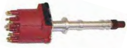
18-5484-1 ELECTRONIC DISTRIBUTOR (Late HEI) Replaces: Mallory YLE624AV For Left Hand Rotation V8/RH 262-454 & 502 (Except 348/409 and Tall Block Engines) • Designed as a plug-in replacement for GM-style fuel ignition system distributor
