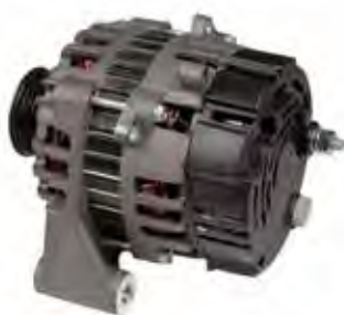
18-5882 ALTERNATOR Replaces: 3884950 75A, 12V, Serpentine 3.0L, 4.3L, 5.0L, 5.7L, 8.1L (2007 - Current)
