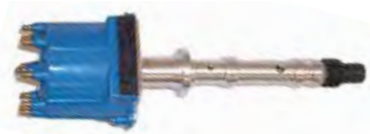
18-5485 ELECTRONIC DISTRIBUTOR (Late HEI) Replaces: Mallory YLE624BV For Right Hand Rotation V8/RH 262-454 & 502 (Except 348/409 and Tall Block Engines) • Designed as a plug-in replacement for GM-style fuel ignition system distributor
